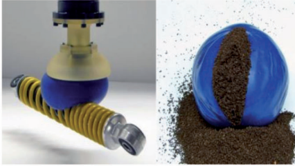
Figure 4. Tool gripper with coffee grounds
