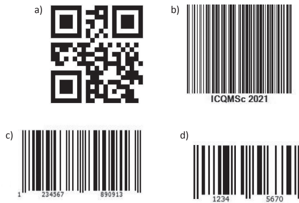
Figure 2. Examples of a two dimensional QR code a) and one dimensional barcodes: Code-128 b), EAN-13 c) and EAN-8 d)
