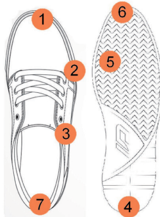
Figure 2. The most common areas of damage to skateboard footwear
